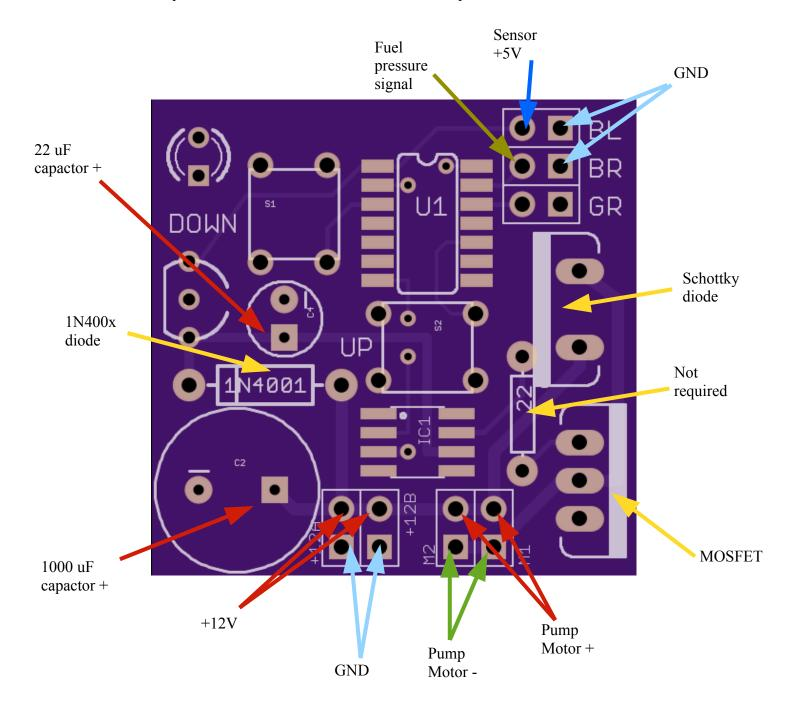
Note polarization of electrolytic capacitors and 1N400x diode. Follow silk screen orientation for power components (heat sink tab is prominent). An image of a completed board can be found at http://www.madhu.com/content/Main/FuelPumpController
